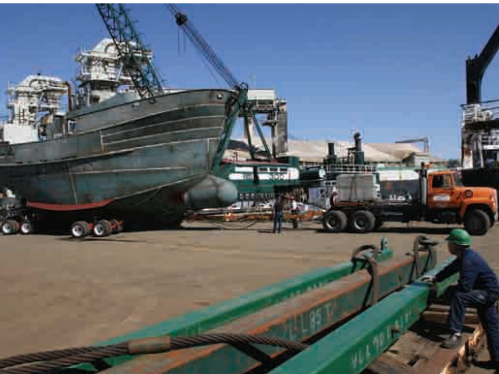
The barge OB-5 is moved into drydock after undergoing replacement of about 90 percent of its bottom plating at Foss Terminal.
