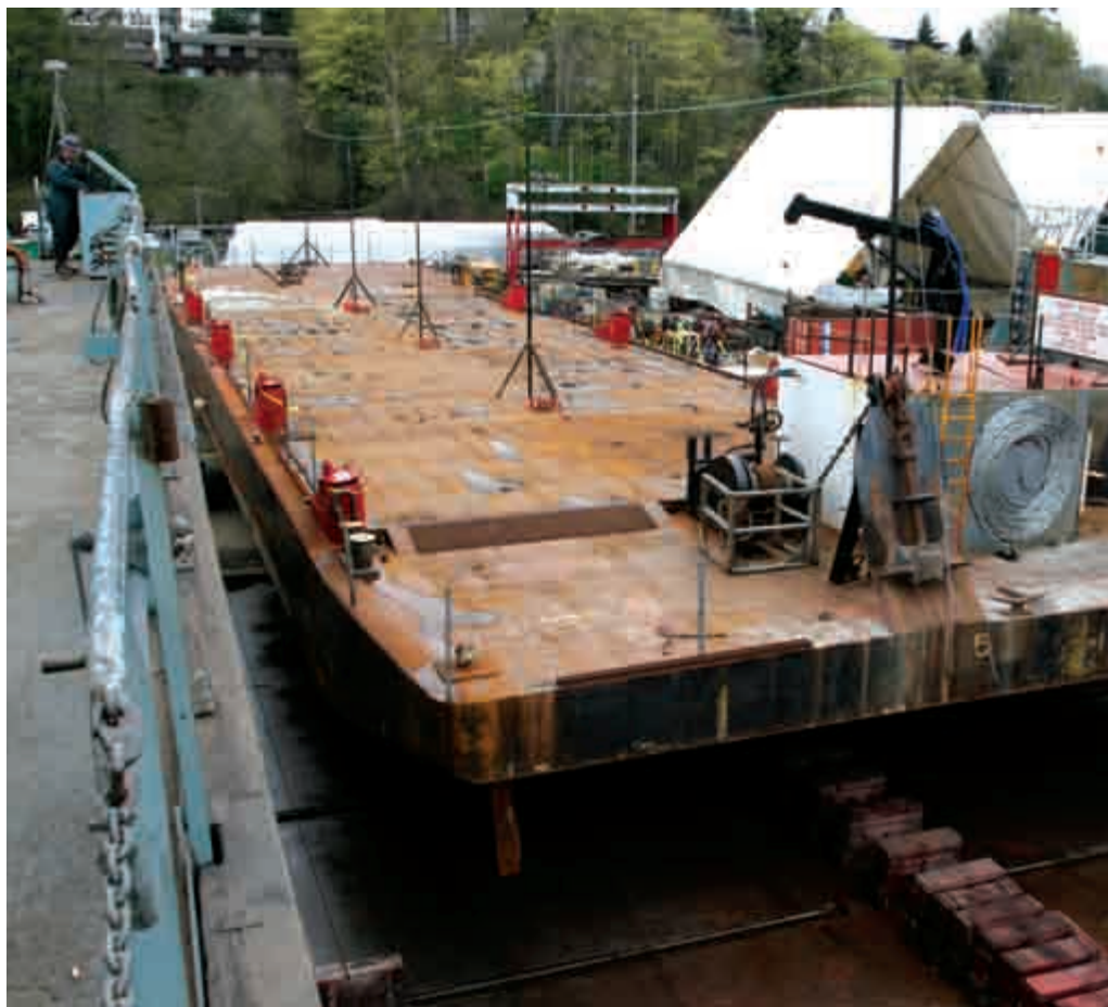
The barge OB-5 is moved into drydock after undergoing replacement of about 90 percent of its bottom plating at Foss Terminal.
