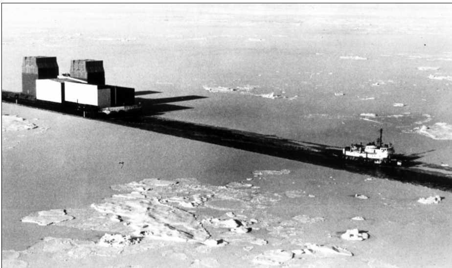
The Arthur Foss tows a module through a narrow channel in the unseasonably heavy ice.
