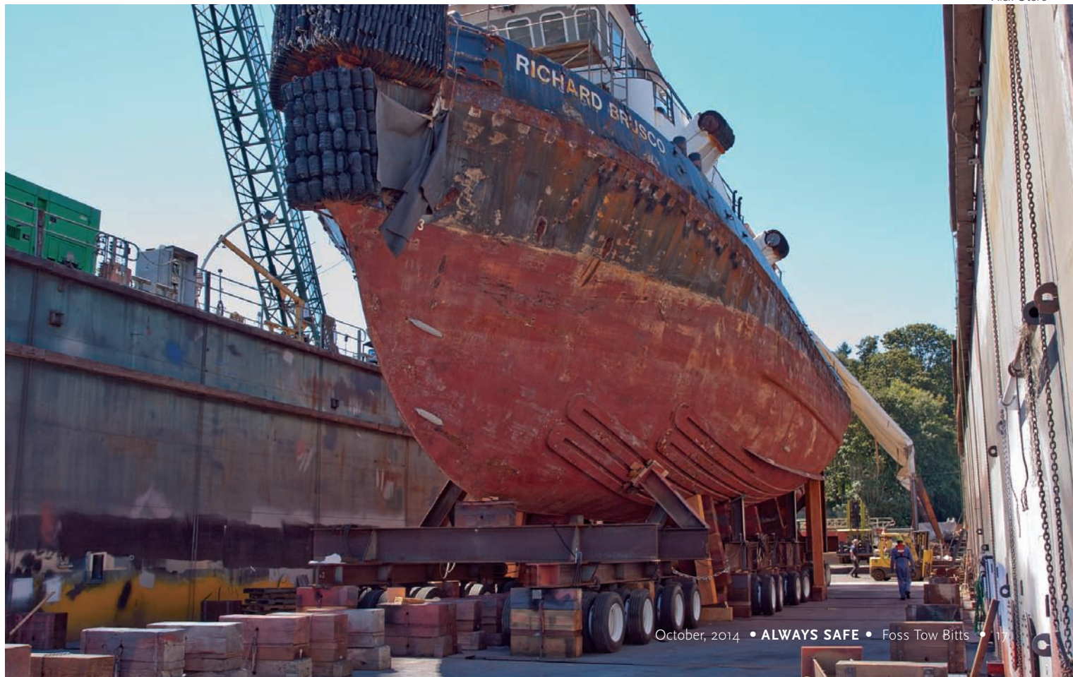
The tug Richard Brusco , being rolled out of drydock and under a tent for extensive repairs.
