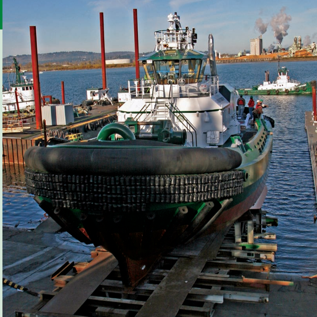
The world’s first hybrid-powered tug, the Carolyn Dorothy , before its launching in 2008 at Foss Rainier Shipyard
