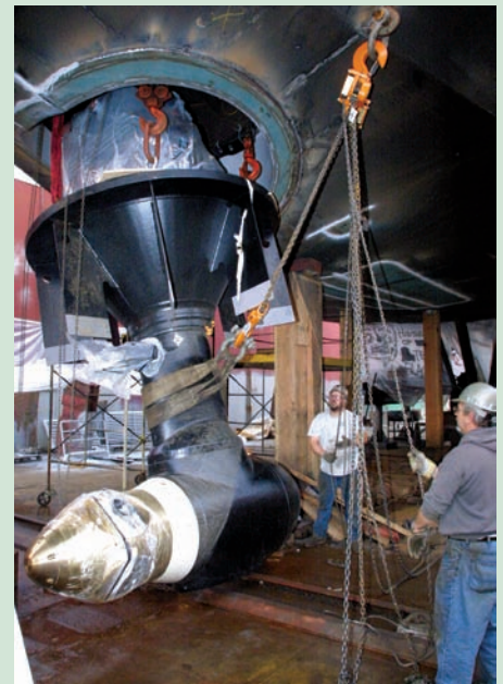
Foss Shipyard in 2007 installed a third propulsion unit on the Brynn Foss , one of three company tugs to be elevated to “Tractor-Plus” status.
