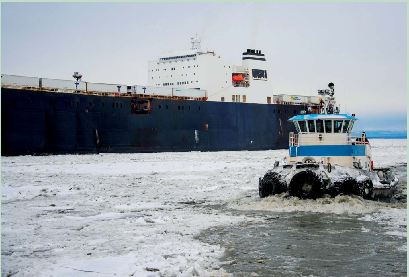
A PATH THROUGH THE ICE The Stellar Wind, operated by Cook Inlet Tug & Barge (CITB), follows a path through the ice carved by a lead tug after they assisted the TOTE ship Midnight Sun at the Port of Anchorage. The ice-class Stellar Wind is 85 feet long and is rated at 3,500 horsepower. CITB is a wholly-owned subsidiary of Foss Maritime. Photos of Foss tugs assisting the Midnight Sun on the other end of its run, at the Port of Tacoma, appears on pages 8 and 9.
