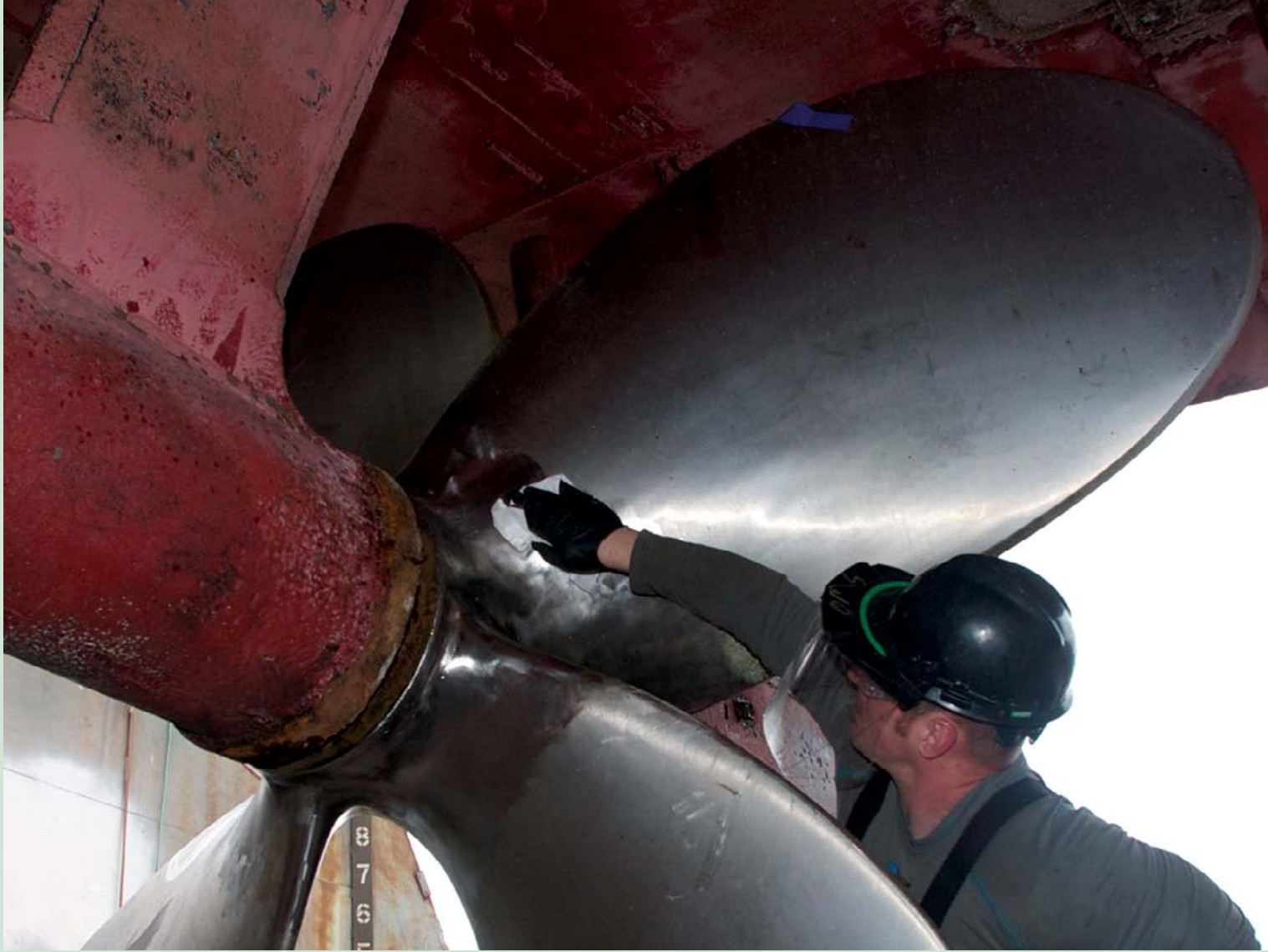
WHEEL WIPING Casey Cheslak, a Foss Seattle Shipyard mechanic, cleans up the starboard propeller of the tug Polar Ranger to check for cracks. The 126-foot, 4,900 horsepower tug is owned by Dunlap Towing of LaConner, Wash., and was in drydock for routine maintenance.
