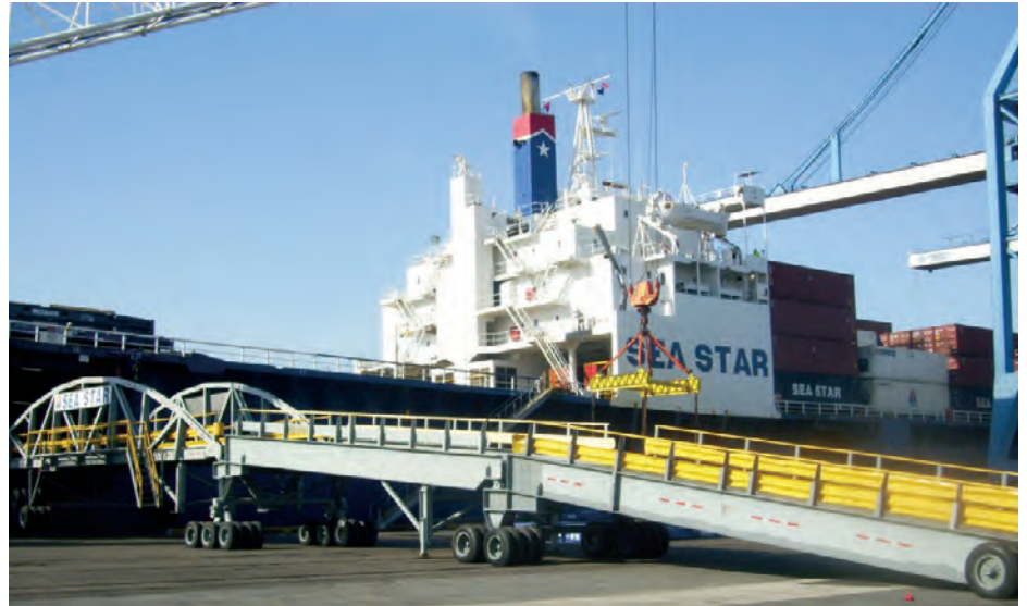
Sea Star's Ponce Class ships are capable of handling both lift-on-lift-off and roll-on-roll-off cargoes simultaneously.
