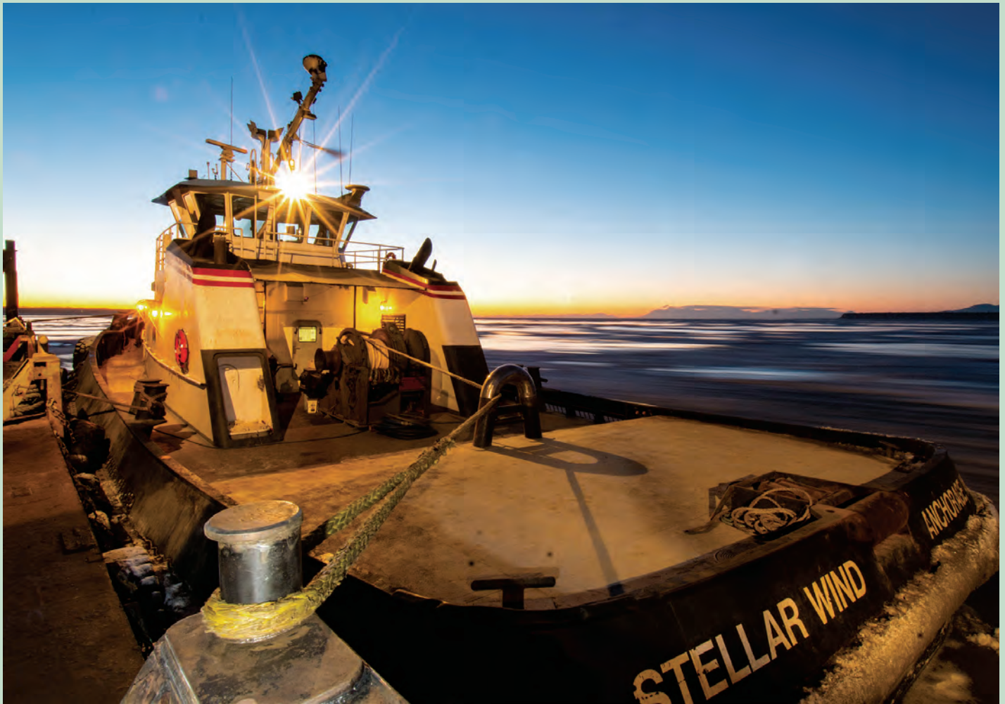
SUNSET IN ANCHORAGE The tractor tug Stellar Wind was photographed at the Cook Inlet Tug & Barge (CITB) float in Anchorage just before a recent sunset. The ice-class tug is 85 feet long and is rated at 3,500 horsepower. It is one of two tractor tugs operated by CITB, which is a wholly owned subsidiary of Foss Maritime.
