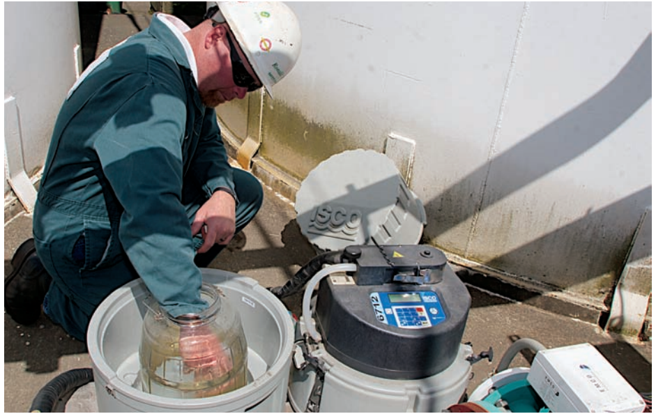
Safety and Health Manager Ron Sykes takes a sample of stormwater collected in above ground tanks. The sample will be forwarded to a lab to be tested for zinc and copper.
