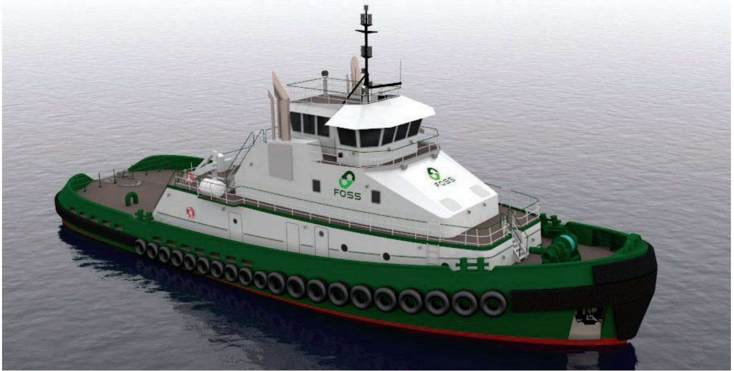
The new Arctic Class tugs, shown here in a computerized rendering, will be 132 feet long and will have ice-strengthened hulls.
