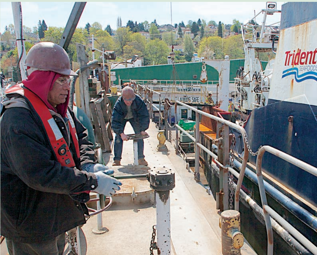
Humberto Moereno , foreground, and Larry Hurtt close drydock valves after bringing up a Trident fishing ship recently.
