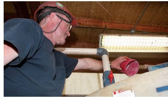
Shipyard Labor Foreman Larry Hurtt adds chemicals to tanks holding drydock wash water that bind and bond heavy metals that are collected as a sediment for disposal.
