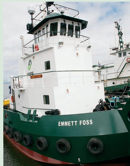
The Emmett Foss is 73 feet long and draws just 3.2 feet, making it ideal for landing barges on Arctic beaches.
