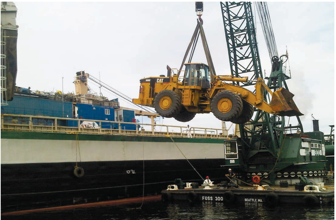
The Foss 300 derrick lifted a one of Foss' existing Red Dog loaders onto the ore barge Kivalina recently at Foss Terminal in Seattle. The Red Dog team this season will be testing new loaders that are 60 percent lighter and use 60 percent less fuel.
