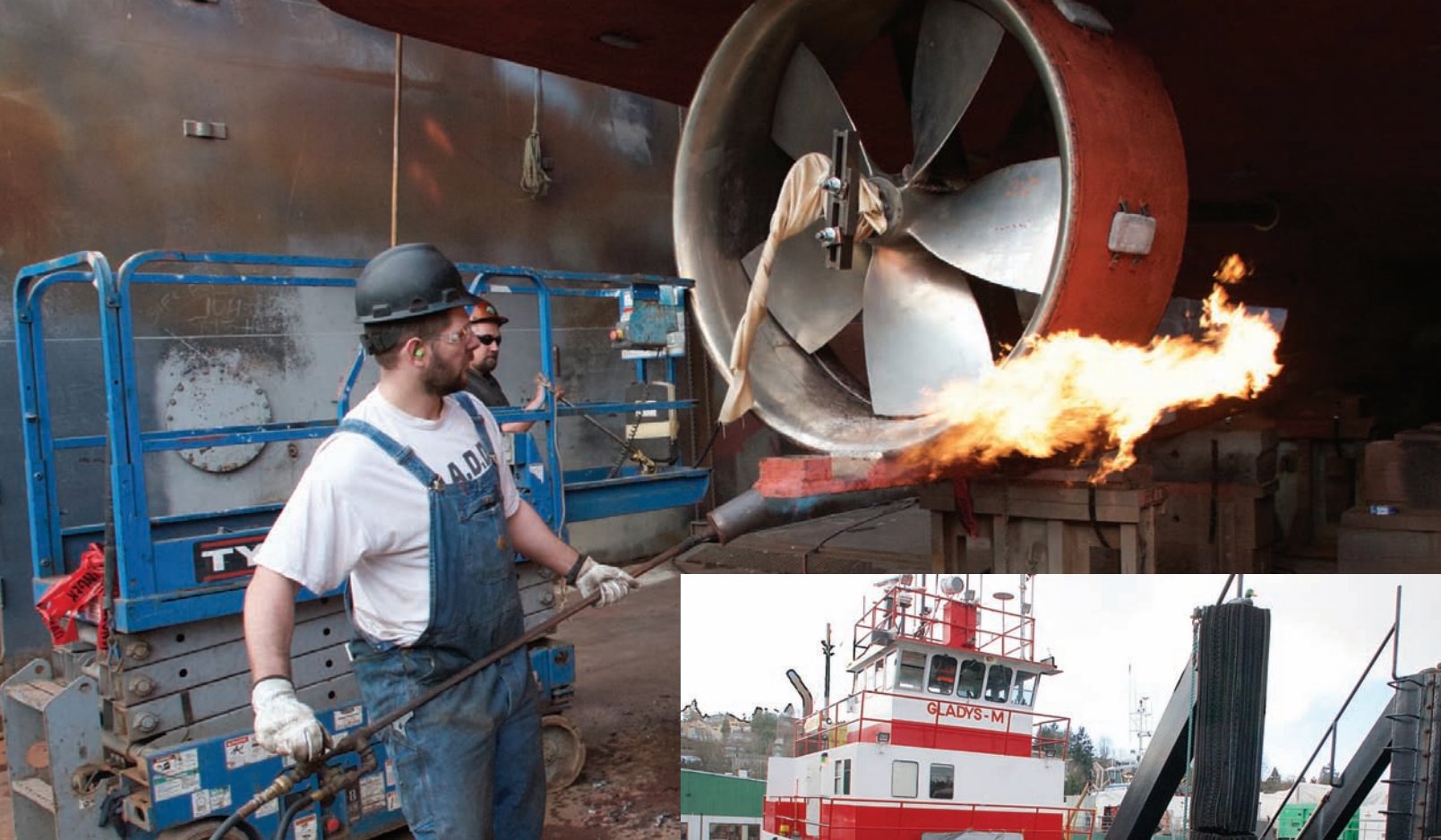
TORCHING THE PROP The Manson pusher tug Gladys M was in drydock at Foss shipyard recently for maintenance work. In the photo above, Machinist Chris Corgain gets ready to heat up the propeller hub, enabling removal of the propeller from its shaft. Beside him is Machinist John Stasiak.
