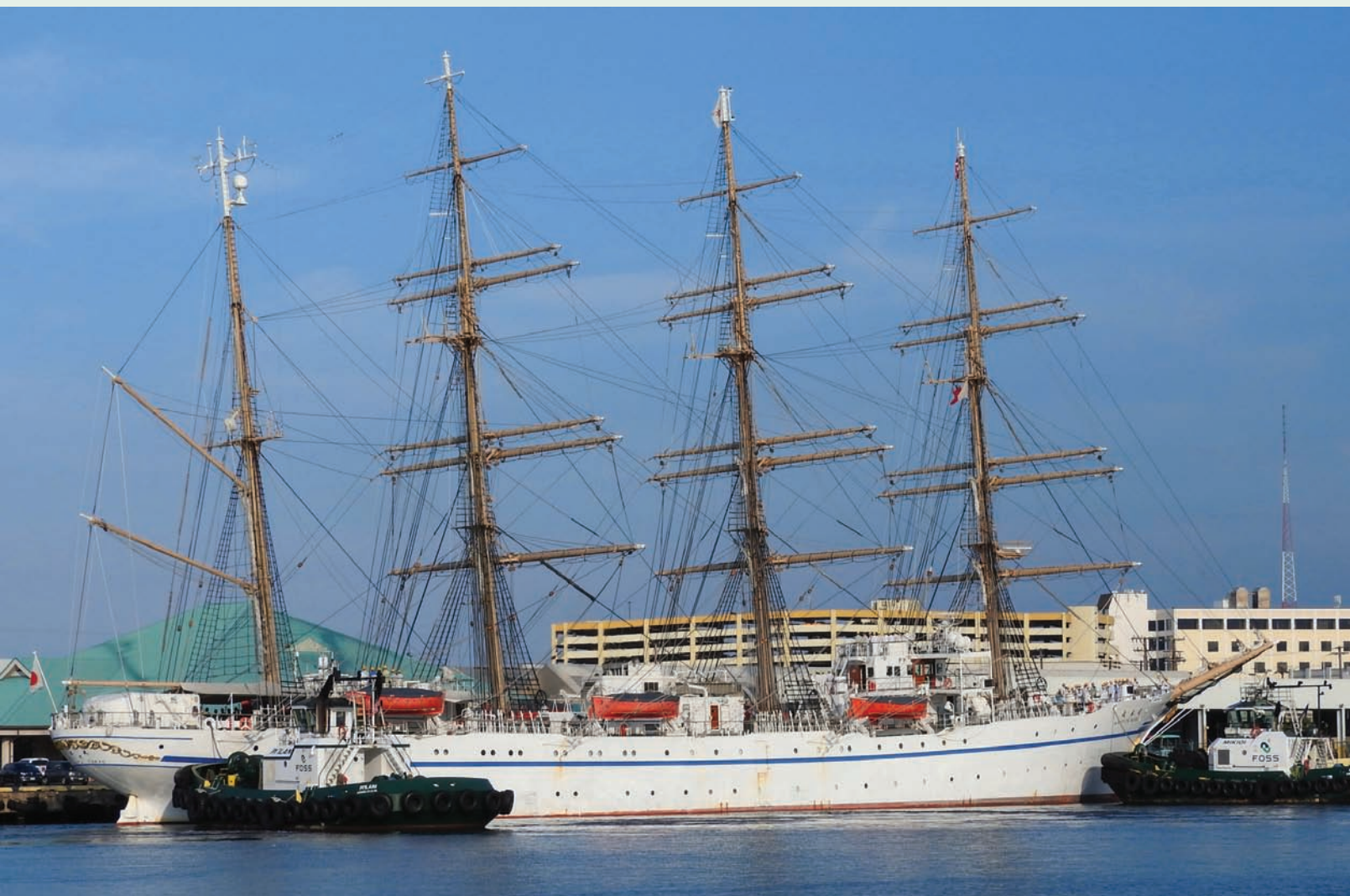
TALL SHIP BACK IN HONOLULU The Foss tugs Mikioi and Piilani assisted the Japanese training ship Nippon Maru into Pier 19 at the Port of Honolulu in late December. The ship, which makes goodwill stops during its training voyages, is a four-masted barquentine, 371 feet long and with a beam of 43 feet. It carries 111 cadets and 60 crew and officers.
