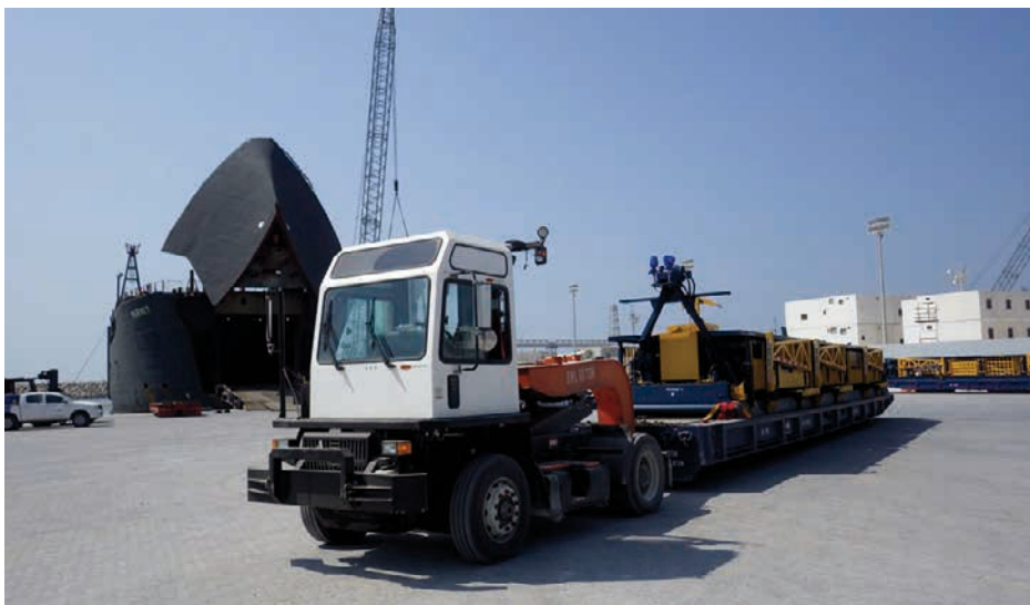
In the photo above, local tugs assisted the Mariner , the barge section of the Strong Mariner , as cargo was offloaded at one of the man-made islands off the coast of Abu Dhabi. Below, cargo was unloaded from the barge on one of the MAFI trailers that carried the rig modules all the way from China.
