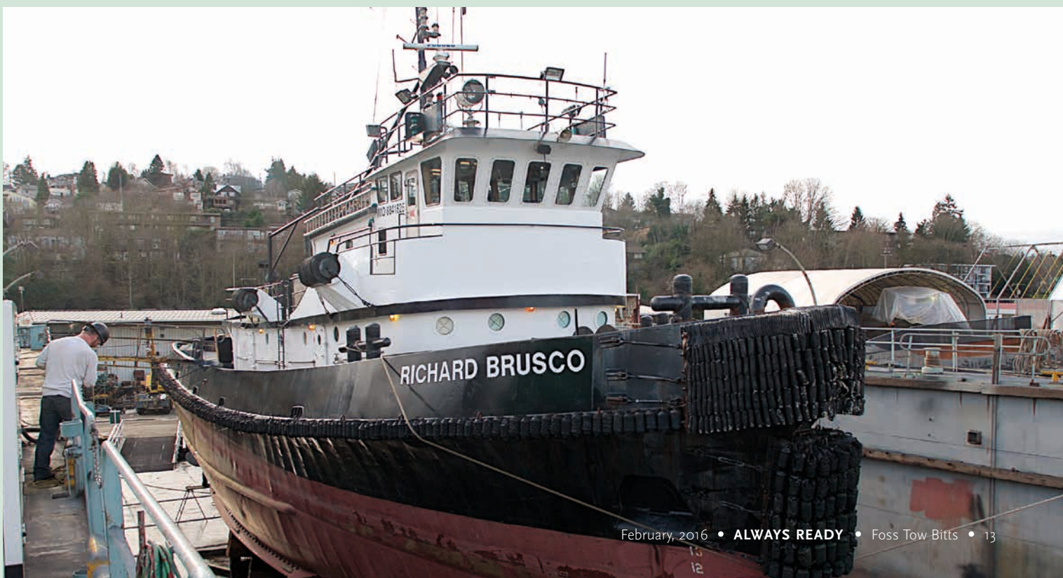
RICHARD BRUSCO IN DRYDOCK Machinist Mark Vandenberg, above, begins the process of removing the port propeller from the tug Richard Brusco, the latest in a series of Brusco tugs to be serviced at Foss Shipyard in Seattle. The propellers of the 112-foot tug were to be tuned up by a contractor, its tow pins were being rebuilt, and it received some touch-up paint.
