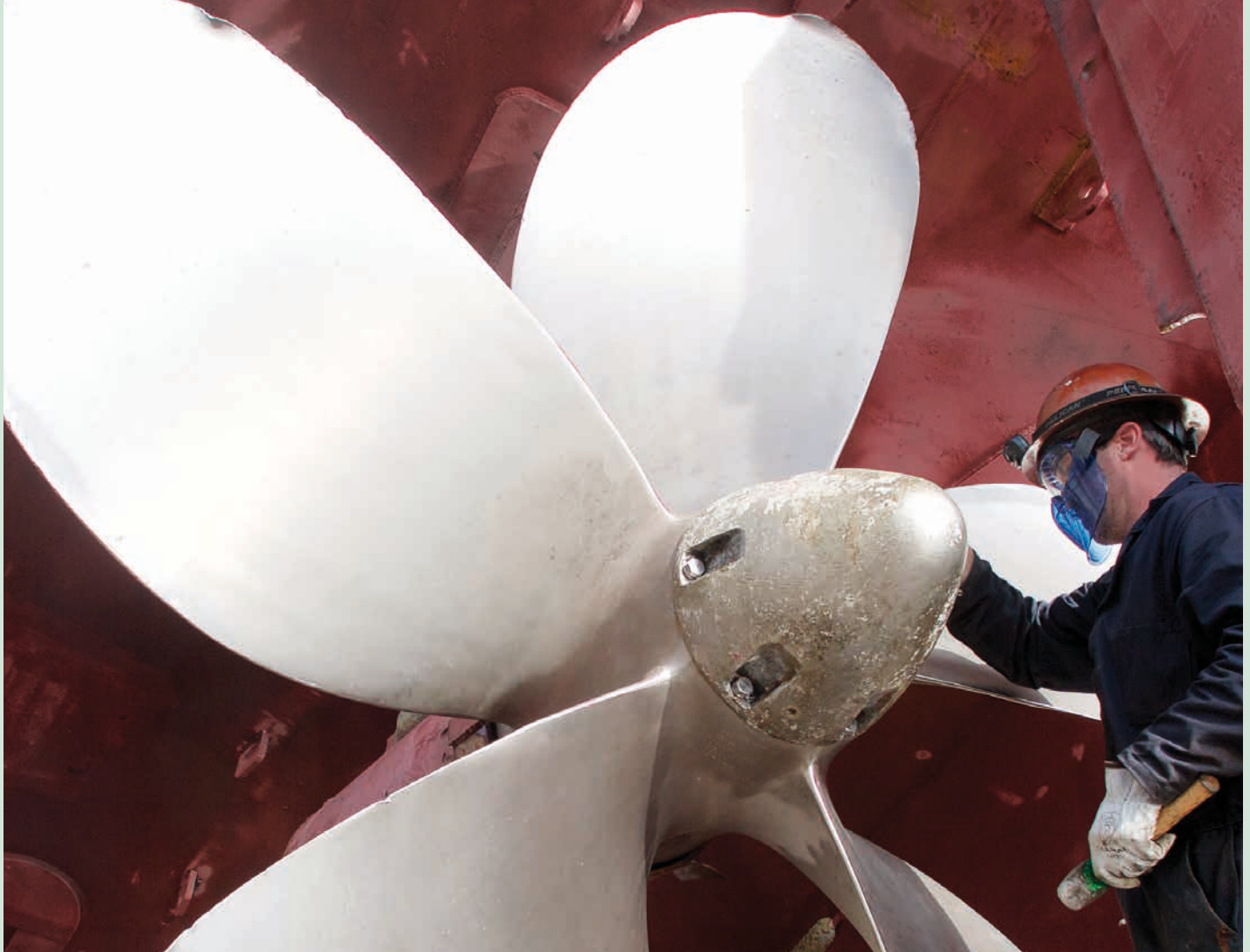
RICHARD BRUSCO IN DRYDOCK Machinist Mark Vandenberg, above, begins the process of removing the port propeller from the tug Richard Brusco, the latest in a series of Brusco tugs to be serviced at Foss Shipyard in Seattle. The propellers of the 112-foot tug were to be tuned up by a contractor, its tow pins were being rebuilt, and it received some touch-up paint.
