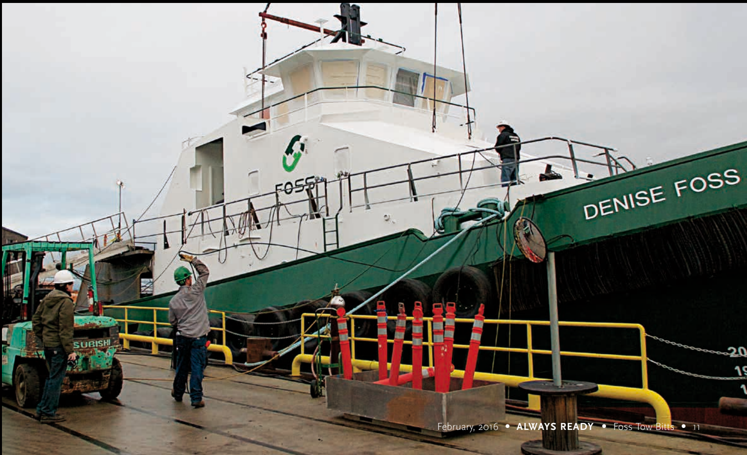
▲ Above: Cook eyeballs the aft end of the house as it is lowered into place.
