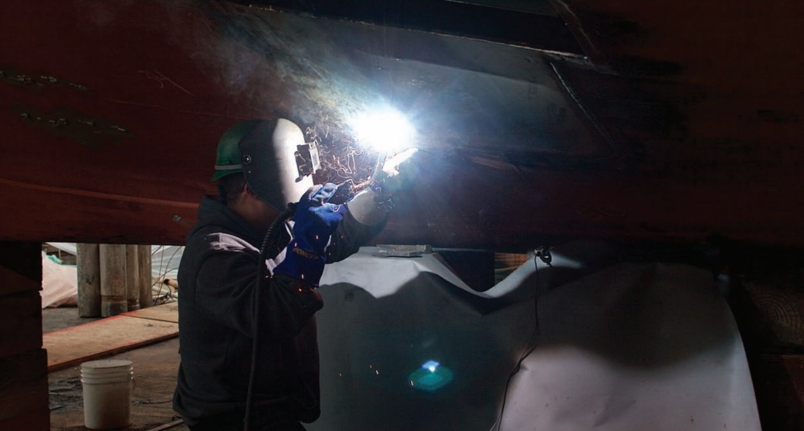
DRYDOCKED IN SEATTLE Foss Seattle Shipyard welder Trevor Abeel works on the hull of the pusher tug Harry M, a Manson tug in dry dock for maintenance. The tug is 104 feet in length and has a beam of 32 feet. The tug is draped in plastic sheeting, standard procedure to protect the environment while vessels are in drydock.
