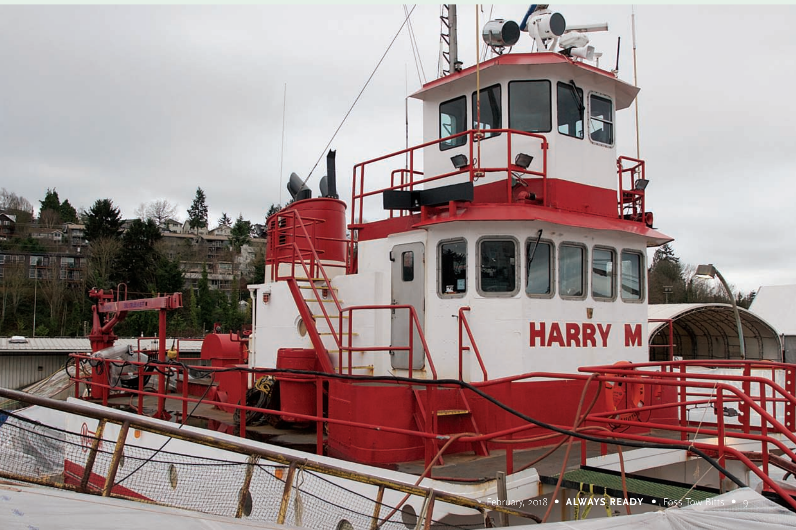
DRYDOCKED IN SEATTLE Foss Seattle Shipyard welder Trevor Abeel works on the hull of the pusher tug Harry M, a Manson tug in dry dock for maintenance. The tug is 104 feet in length and has a beam of 32 feet. The tug is draped in plastic sheeting, standard procedure to protect the environment while vessels are in drydock.
