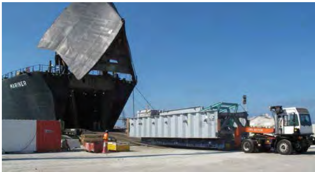
Cargo comes off the Mariner through its clamshell bow.
