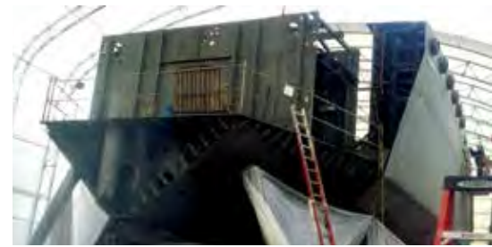
The first of three Arctic Class tugs takes shape at Foss Rainier Shipyard. Delivery is scheduled for late this year. The vessels will be 132 feet long and will have ice strengthened hulls. Jerome Ruhoff
