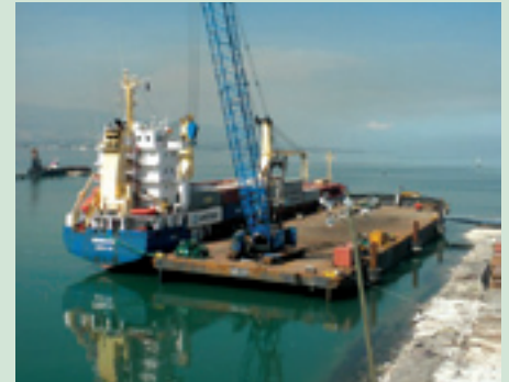
A cargo ship is alongside the newly-placed barge Columbia Boston , serving as a temporary pier in Port au Prince.
