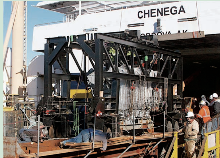
Shipyard workers rolled the first of four engines, at 15 tons, out of the Chenega .
