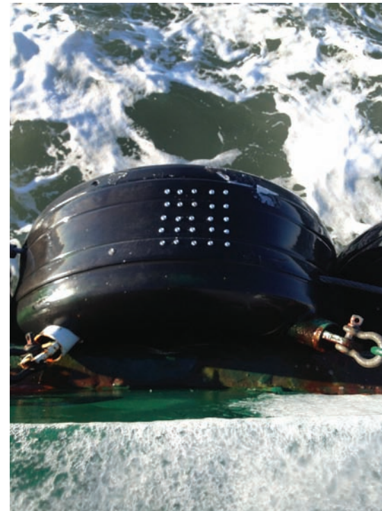
The screws drilled into the tires have raised heads, improving safety in icy weather.
