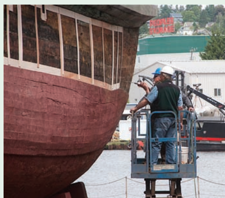
Surveyors drilled into the tug's hull, looking for soft spots in planks that might need to be replaced.
