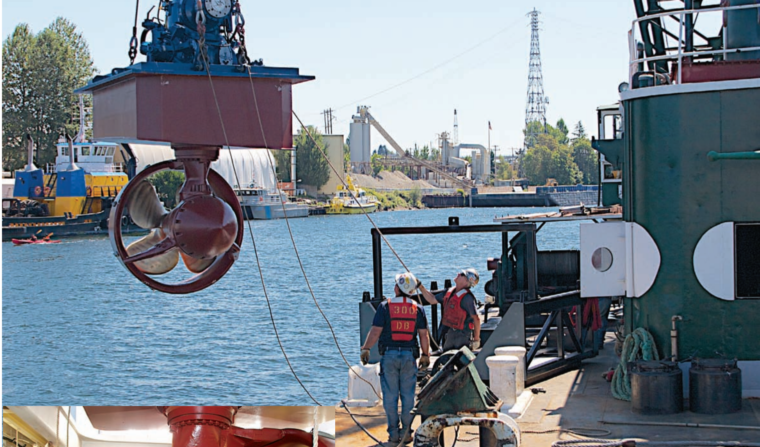
Z-DRIVE INSTALLATION In the photo above, Foss 300 derrick Operator John Tarabochia left, looked on and Rigger Jim Fox handled the tagline as the derrick lifted the second of two 12-ton Z-drives toward the Coast Guard Buoy Tender Anthony Petit , in drydock. In the photo at left, Machinist Brian Anderson guides the drive into the engineroom. Installation of the drives was a major portion of the work on the 175-foot vessel, homeported in Ketchikan, Alaska.
