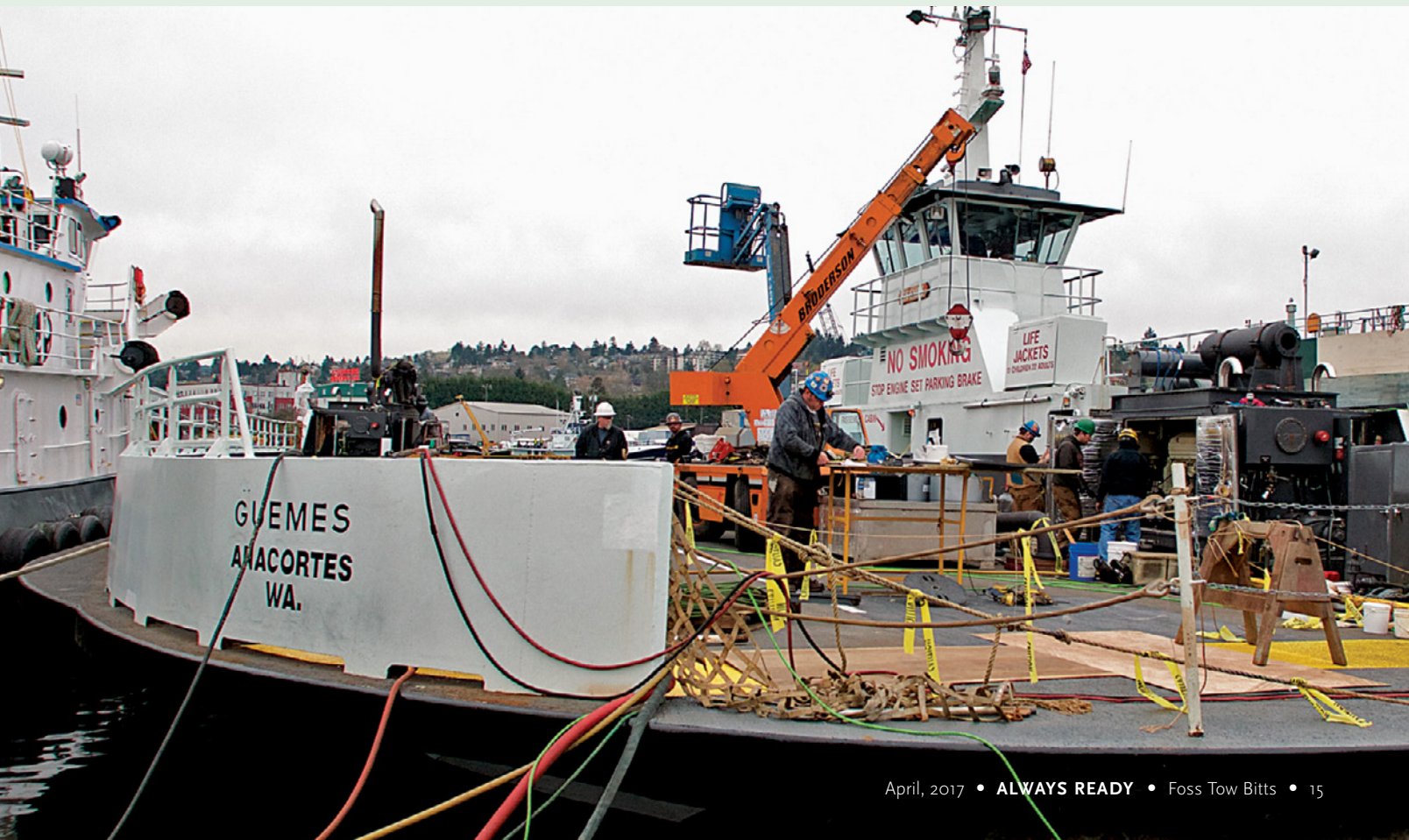
CHECKING AND WELDING Foss Shipyard welder Simon Izotov checked the fit of an engine bed bracket and then welded the bracket into place recently at the yard. The engine bed belongs to the 21-vehicle ferry Guemes , below, which is operated by Skagit County between Guemes Island and Anacortes, Wash. The ferry was drydocked at the yard in March for extensive maintenance.
