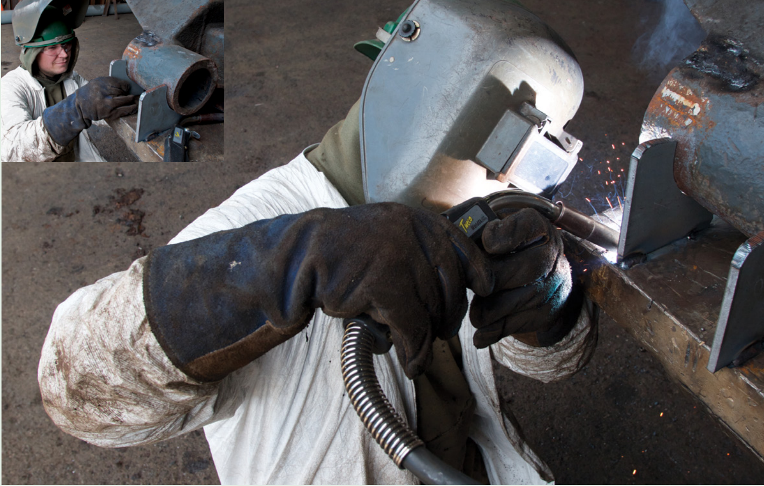
CHECKING AND WELDING Foss Shipyard welder Simon Izotov checked the fit of an engine bed bracket and then welded the bracket into place recently at the yard. The engine bed belongs to the 21-vehicle ferry Guemes , below, which is operated by Skagit County between Guemes Island and Anacortes, Wash. The ferry was drydocked at the yard in March for extensive maintenance.
